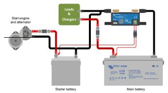
Measuring voltage of the starter battery
