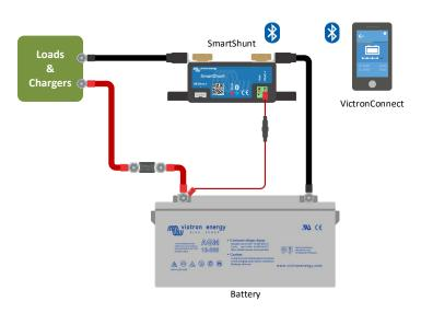
Basic SmartShunt wiring
