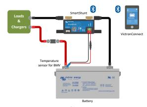
Measuring battery temperature
