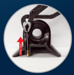
Remove the faulty valve: Screw a 3mm screw inside the centre of the valve and pull it out with a tong (tool).
