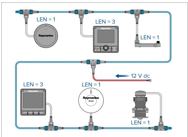
In the example above the backbone has an overall LEN of 10, so the optimum connection point would be to have 5 LEN either side of the connection point.
