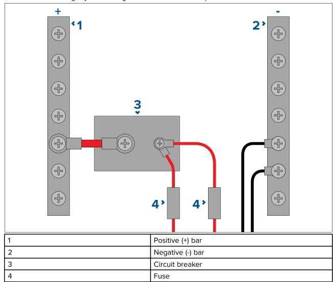
Where possible, connect individual items of equipment to individual circuit breakers. Where this is not possible, use individual in-line fuses to provide the necessary protection.
