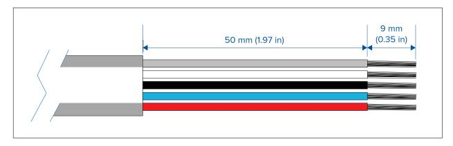
2. Fit each wire into the corresponding color coded connector. To fit the wires use a flat blade screw driver to push in the spring retention clip and hold it in the open position, then slide the wire fully into the connector and release the spring retention clip.
