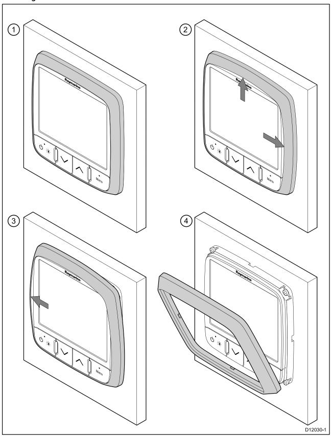
**Important:** Take care when removing the bezel. Only use a plastic pry tool (not supplied) to lever the bezel, attempting to use another tool may cause damage.
