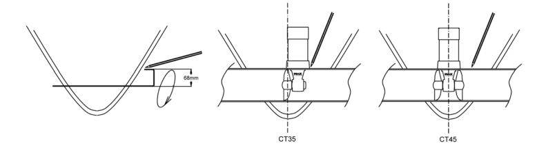
Replace the tunnel. To secure its position apply reinforced fibreglass filler to all areas, both inside and out, taking care to entirely fill the space between the hull and the tunnel. Laminate using a minimum of 8 layers of **ISOPHTALIC RESIN** alternated with mat and roving.
