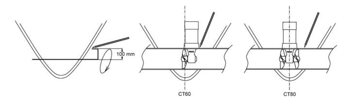
Replace the tunnel. To secure its position apply reinforced fibreglass filler to all areas, both inside and out, taking care to entirely fill the space between the hull and the tunnel. Laminate using a minimum of 8 layers of **ISOPHTALIC RESIN** alternated with mat and roving.
