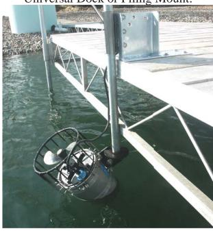
Kasco's heavy duty dock or piling mount is made from corrosion protected steel and stainless steel. This dock mount can be used with any of our de-icer units. Users supply their own 10 foot 1" O.D. pipe. Includes a Qwiklock handle for easy installation and adjustments
