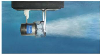
The horizontal float is an easy to assemble kit consisting of stainless steel components and a flotation block. The de-icer is mounted at an angle just below the float producing an elongated pattern of agitated water and is well suited for shallow water operation.
