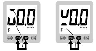
Figure 9 - Switching Between Surface and Keel Depth.
