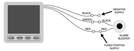
Figure 1 - Echosounder and Alarm Bleeper Connections
