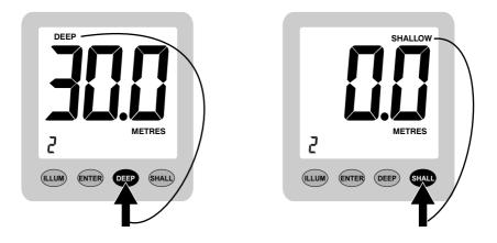
Figure 6 - Selecting Deep or Shallow Alarm Setting
