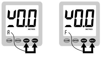
Figure 11 - Switching Between Averaged and Fast Display Modes
