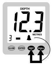
Figure 7 - Activating and de-Activating the Alarms
