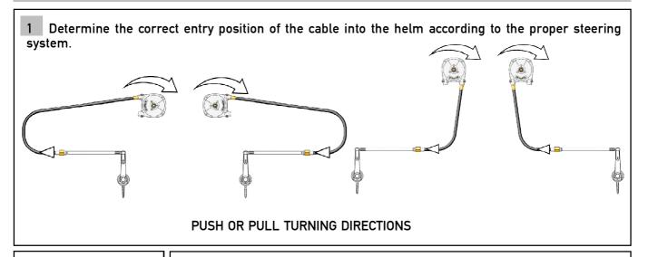
2 Remove protective pipe from cable **ULTRAFLEX** M66 and insert the helix cable into the helm.
