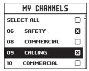
Subsequent opening of this page will show a list of only the selected channels. Choosing one of the channel options immediately exits the page and sets the radio to that channel.
